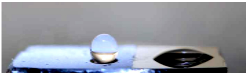
Fig. 1 Superhydrophobic coating. (Reproduced with permission from Ovaskainen, L., et al., Superhydrophobic polymeric coatings produced by rapid expansion of supercritical solutions combined with electrostatic deposition (RESS-ED) , J. Supercrit. Fluids 95 (2014) 610–617, Elsevier.)
