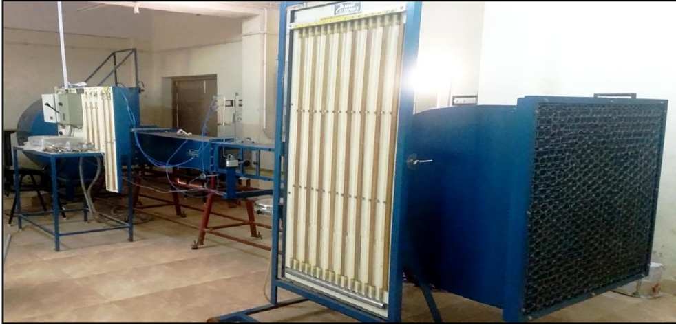
Fig. 18 Computerized low-speed subsonic wind tunnel facility.
